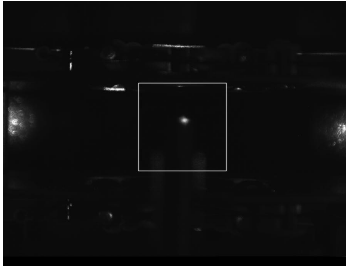
Figure 6.3: Fluorescence image of 3D MOT recorded by a camera behind the science chamber.
