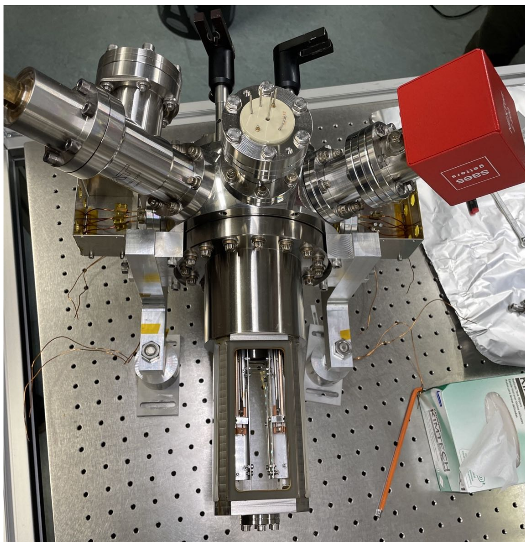
Figure 5.4: Titanium 2D chamber mounted on a stainless steel spherical octagon.
